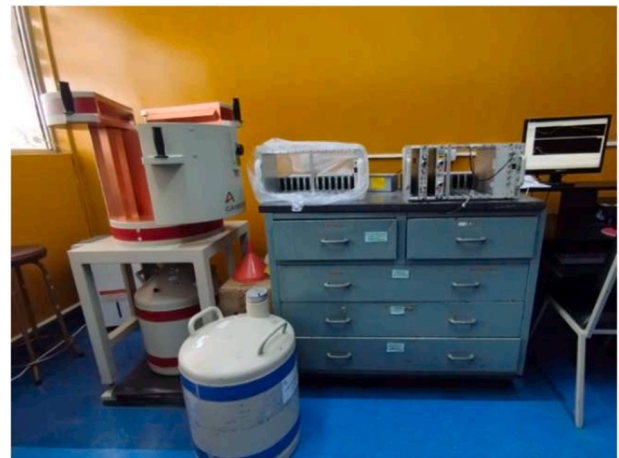
Fig. 2. Chain for gamma spectroscopy with the HPGe detector of 150 % efficiency, together with the shield, its Dewar and electronic chain in the Division of Analytical and Nuclear Techniques of IPEN.
