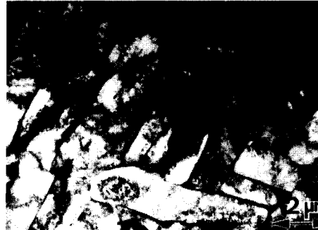
Figure 4-Zr-1.0wt% Nb, heat treated and 5% cold worked. High density of dislocations inside the subgrains (electron micrograph)
