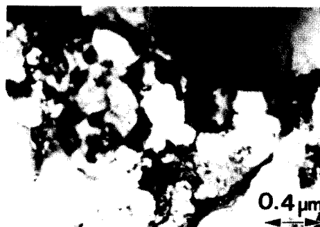
Figure 6- Zr-1.0wt%Nb, 60% cw, heat treated, T=550° C for 1 h. Beginning of the recrystallization; small α-grain (electron micrograph)
