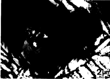
Figure 3-As-cast Zr-0.5wt% Nb, grains of alpha Zr surrounded by beta phase widmannstatten microstructure (electron micrograph)
