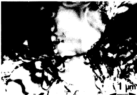
Figure 9- Zr-1.5wt%Nb, 60% cw, heat-treated, T=750° C for 2 h. \alpha -grains; \alpha -transformed by quenching, some number of dislocations (electron micrograph)
