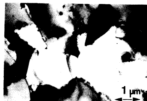
Figure 10- Zr-1.0wt%Nb, 60% cw, heat-treated, t=700° C for 5 h. Typical microstructure of a recrystallization in two phases, \beta -phase growing in a triple junction of \alpha (electron micrograph)
