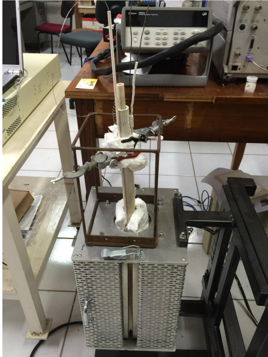
Experimental setup for measuring luminescent emission during electric field-assisted sintering.
