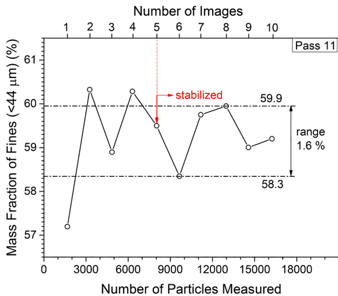
Fig. 12. Influence of the number of processed images on the results of the fine (<44 \mu m ) content determination in the finished fuel plate meat (after rolling pass 11).
