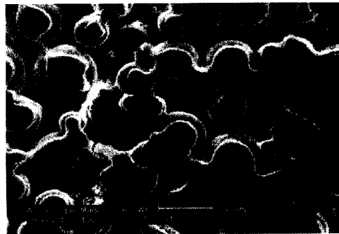
Fig. 6: SEM micrograph of 304L SS filter after surface treatment of 7 days in 3 mol/L \text{H}_2\text{SO}_4 with 0.1 mol/L BTAH followed by immersion for 11 days in 3 mol/L \text{H}_2\text{SO}_4 at room temperature.
