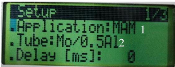
Figure 2: Diavolt menu screen, showing the application (1) and the target-filtration combination (2)
