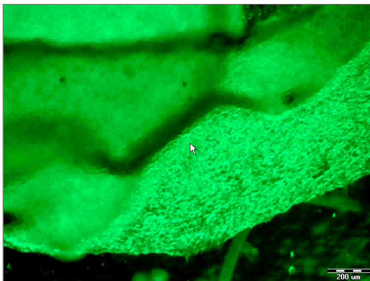
FIG. 13. A snapshot microscope photograph illustrating temperature triggered detachment of a fibroblast cell layer from the radiation synthesized PP-g-TMA surface.
