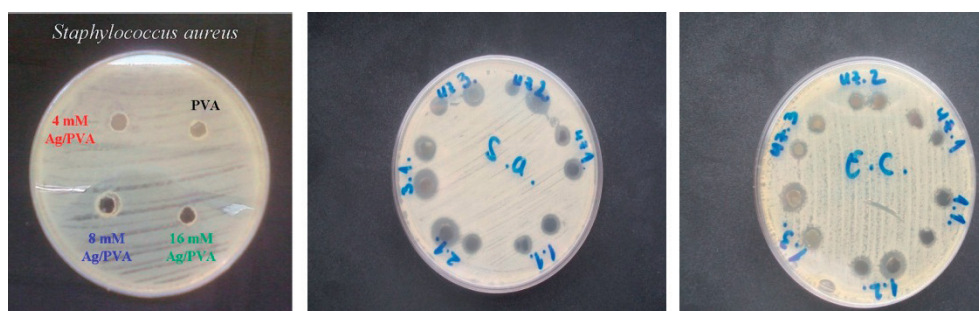
FIG. 8. Serial plate transfer test for S. aureus (centre) and E. coli (right), clearly showing a zone of growth inhibition surrounding the disc with Ag NPs, compared with the control (left).
