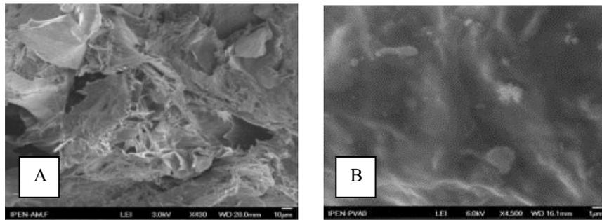
**Fig. 4** - SEM micrographs of lyophilized hydrogels (A) PVAI / 1.0% clay and (B) PVAI / 1.5% clay.
