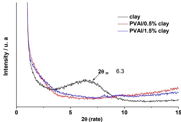
Fig. 2 - XRD curves of hydrogel membranes of PVAL / clay.
