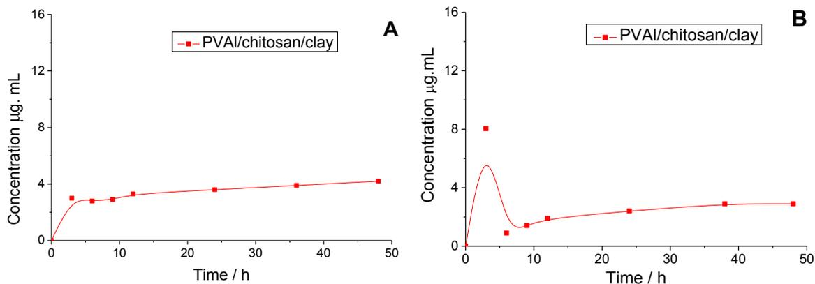
**Fig. 8** - Static curves of the kinetics of release of glucantime hydrogels (A) PVAI / 1.5% clay and (B) PVAI/chitosan/1.5% clay.
