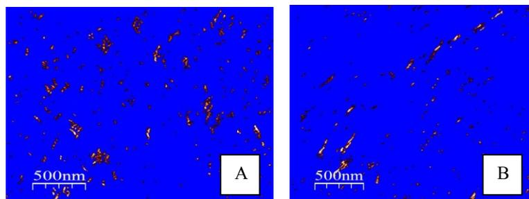
**Fig. 6** - AFM obtained from the sample surface lyophilized hydrogels (A) PVAI / 1.0% clay and (B) PVAI/chitosan/1.0% clay.
