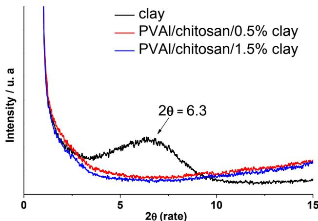
Fig. 3 - XRD curves of hydrogel membranes of PVAL / chitosan / clay.
