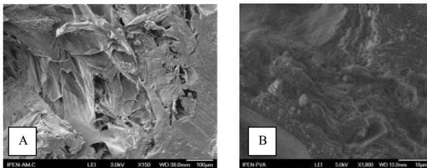
**Fig. 5** - SEM micrographs field emission (SEM-EC) of lyophilized hydrogels (A) PVAI/chitosan/1.0% clay and (B) PVAI/chitosan/1.5% clay.
