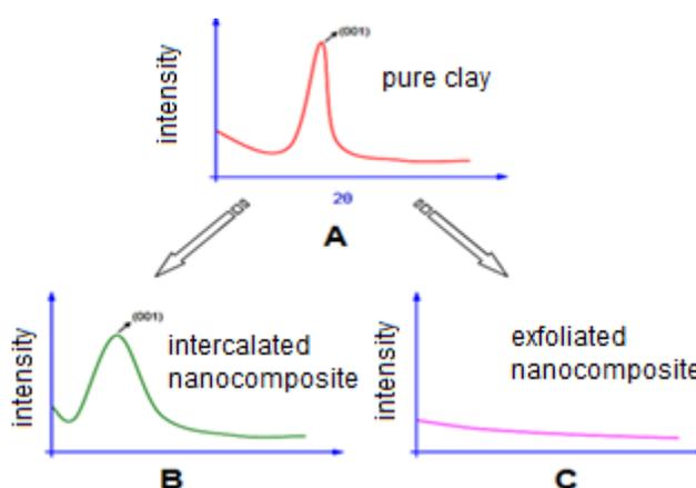
**Fig. 1** - The different representations of the dispersion of the clay in relation to the polymer by XRD analysis (A) pure clay (B) in relation to the intercalated clay and the polymer (C) exfoliated clay relative to the polymer.
