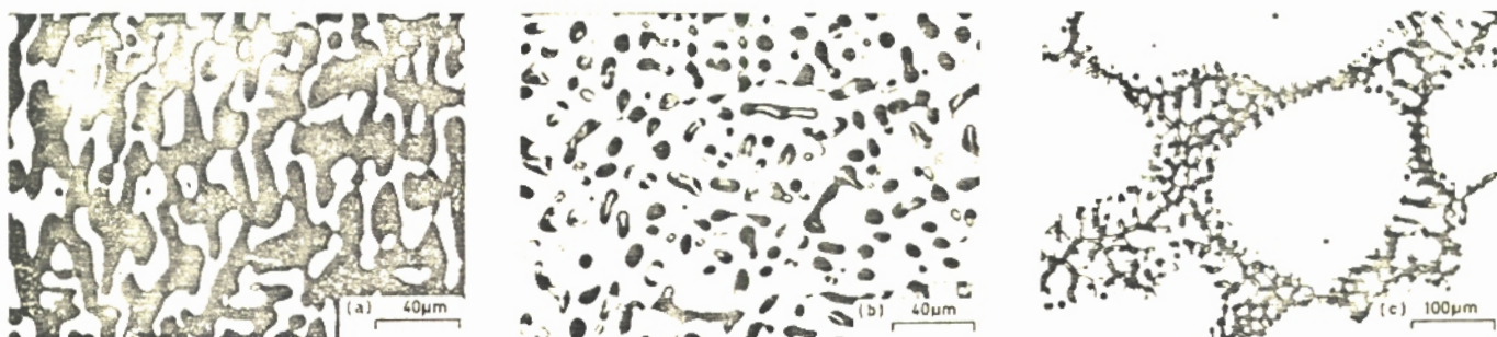
Fig. 5a to c. Microstructures of alloys in the Mo-Rh-Pd system after annealing at 1700 °C. (a) 75 Mo, 5 Rh, 20 Pd (at.%); dark: \beta + \epsilon , bright: \epsilon . (b) 60 Mo, 5 Rh, 35 Pd; dark: \beta , bright: \epsilon . (c) 20 Mo, 30 Rh, 50 Pd; bright: \alpha , dark phases at grain boundaries: liquid.
