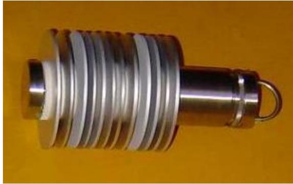
Figure 1. A typical rack with a stack of circular coupons.
