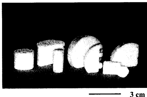
Figure 1. Bioactive 58S sol-gel foams produced in a variety of shapes and sizes.
