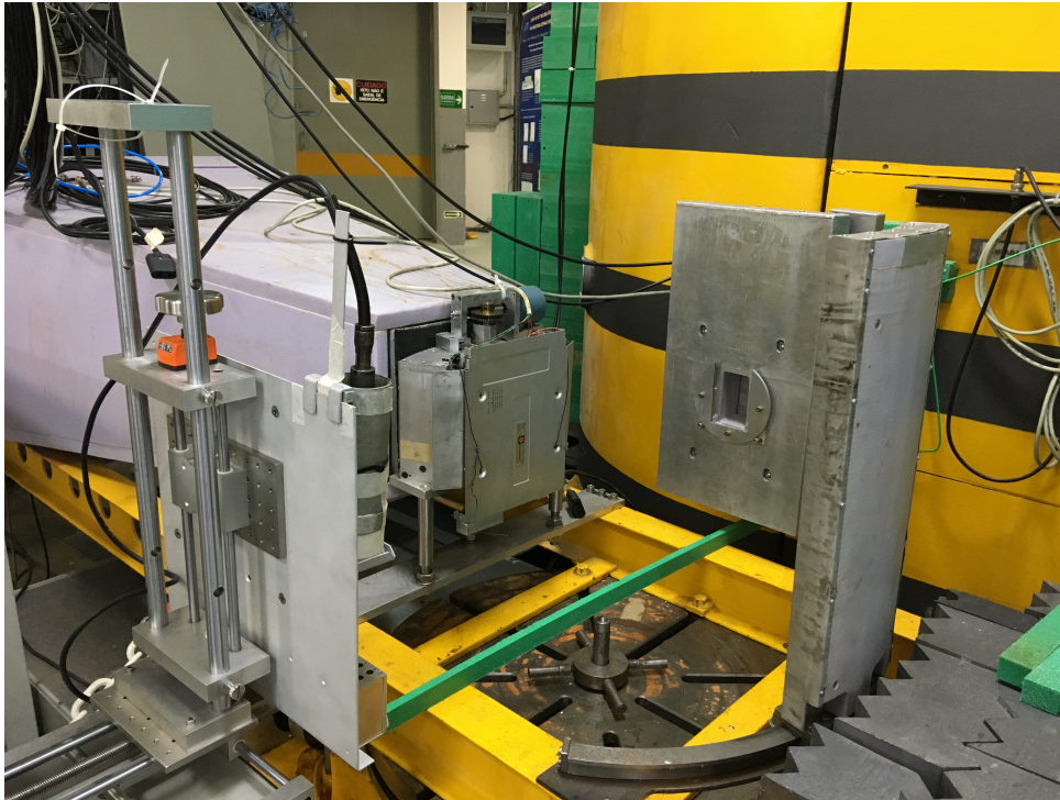
Figure 1. Thermal neutron irradiation setup
