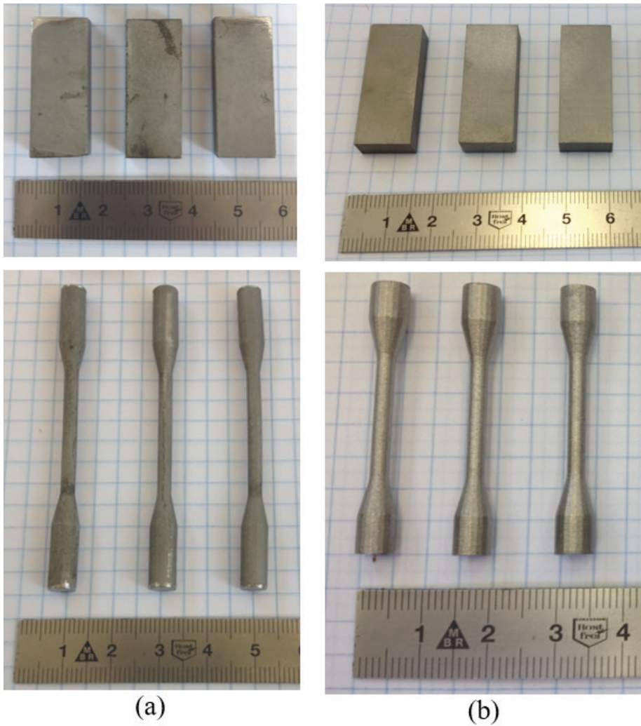
Figure 6. Specimens manufactured of Co-Cr-Mo alloy: (a) specimens made by FP technique and (b) specimens made by SLM technique.
