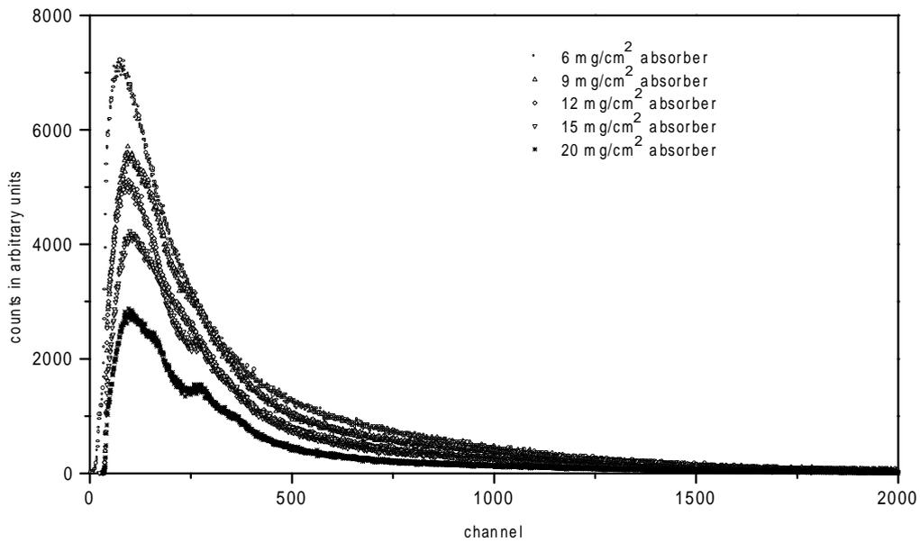
**Figure 2:** Variation of the  $\beta$  detection with the 6 to 20  $\text{mg}/\text{cm}^2$  absorbers.
