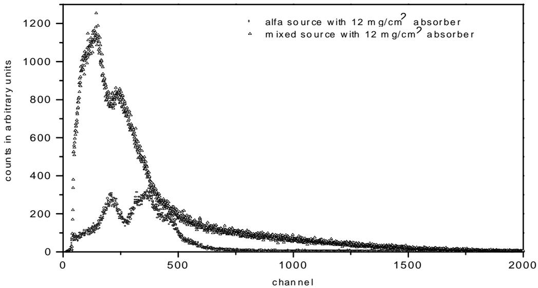
**Figure 3:** Particles detection from mixed and pure  $\alpha$  sources with 12  $\text{mg}/\text{cm}^2$  absorbers.
