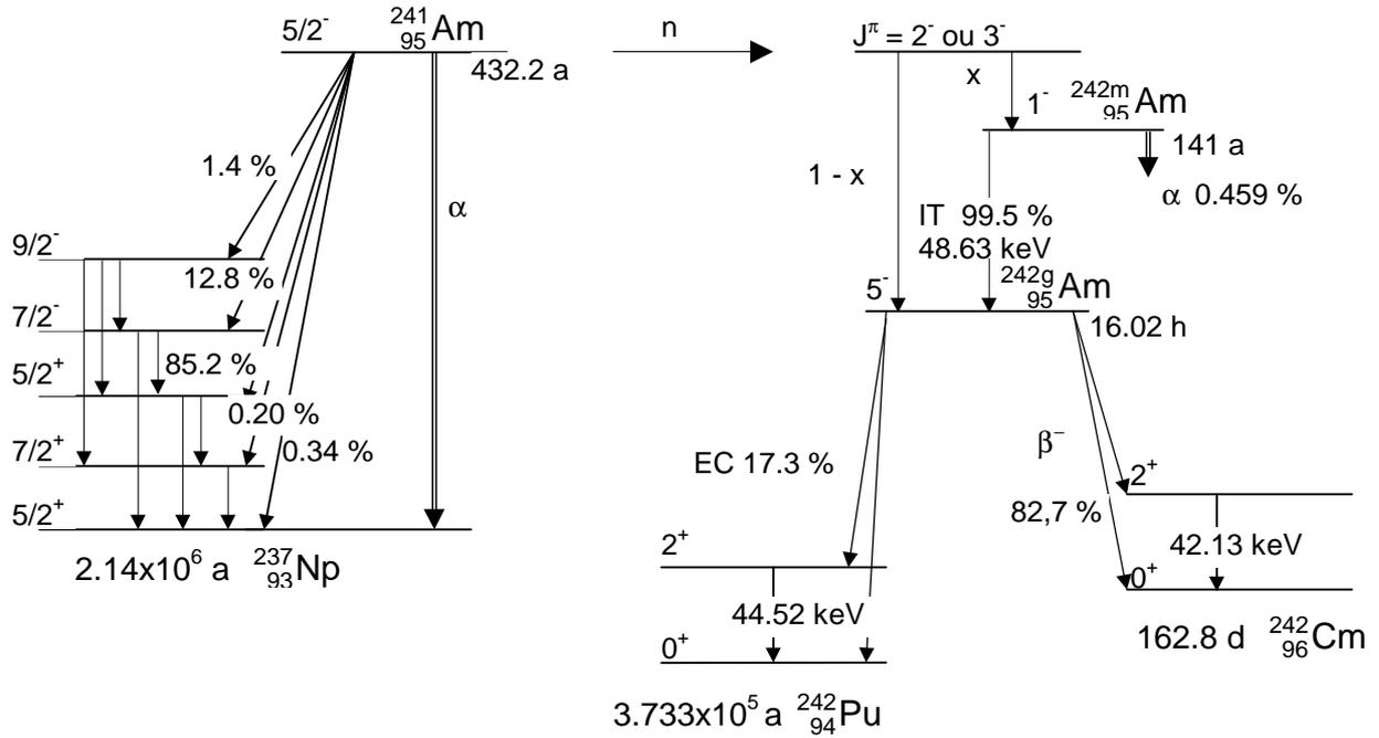
**Figure 1:** Scheme of the  $^{241}\text{Am}(n,\gamma)^{242g}\text{Am}$  reaction [2].
