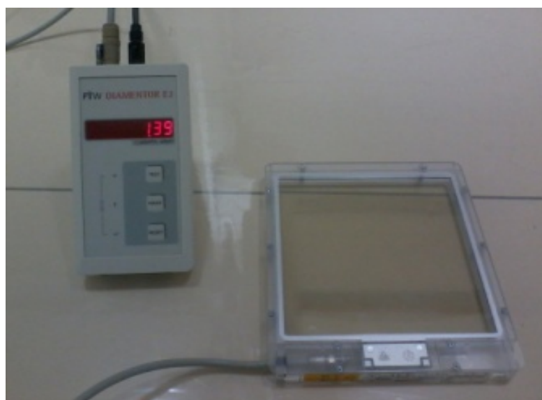
Figure 1. The KAP meter. Left: the reading module. Right: the square chamber.
