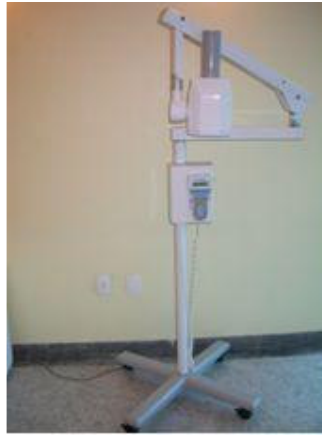
Figure 1. Dental X rays machine, Dabi Atlante, model Spectro 70X Seletronic, Characteristics: 70kVp, 8mA and nominal filtration of 2.71mmAl.
