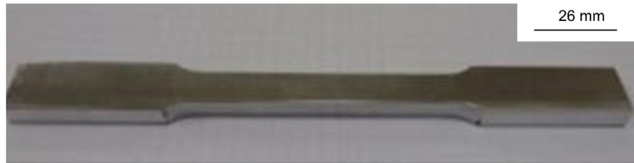
Fig. 2 – Specimen for tensile and fatigue tests machined from extruded profiles of AA7108 and AA7046.
