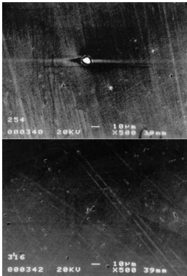
6 Scanning electron micrographs of 254SMO (top) and 316L (below) after polishing with 1 µm diamond paste
