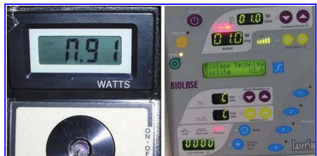
FIG. 3. Power meter showing the PO measured at the optical fiber tip (left). Diode-laser control panel (right) displaying the laser power, which is higher than the PO measured by the power meter at the optical fiber tip.
