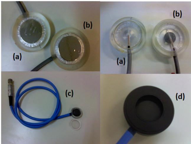
Fig.1. Ionization chambers tested: Homemade parallel-plate chambers with aluminum (a) and graphite (b) collecting electrodes; Advanced Markus chamber(c) and Ross chamber (d).
