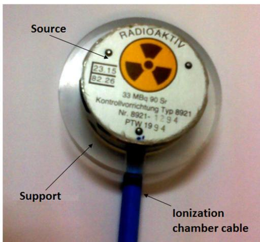
Fig. 2.  $^{90}\text{Sr}+^{90}\text{Y}$  PTW check device at the acrylic support, on the ionization chamber.
