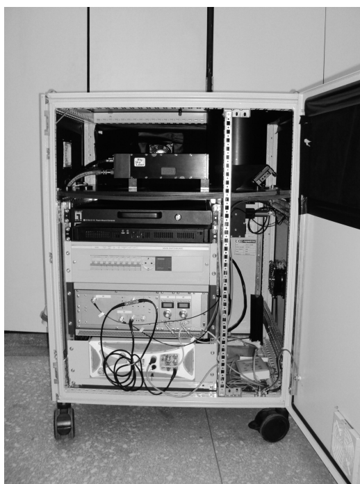
Figure 2: Raymetrics Mobile LIDAR System
