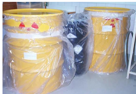
Figure 10. Drums employed for storage of the radioactive wastes generated in the glove-boxes decommissioning operations.
