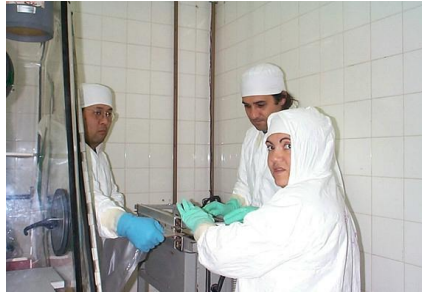
Figure 8. Materials removal from the glove-boxes using the “bag in-bag out” system.
