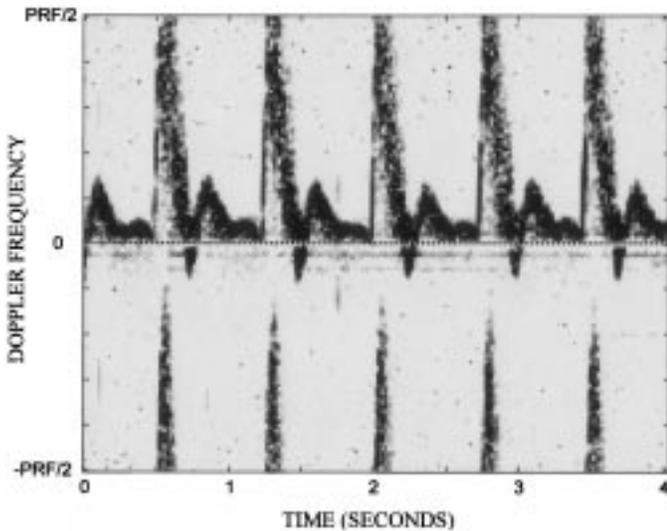
Fig. 5. Spectrogram from a brachial artery of a healthy person, obtained with a conventional PDUV. Positive frequencies represent direct flow and negative frequencies represent reverse flow. The spectral components from direct flow occupy the range  $(-PRF, 0)$ , reserved for reverse flow, clearly indicating subsampled Doppler signals.
