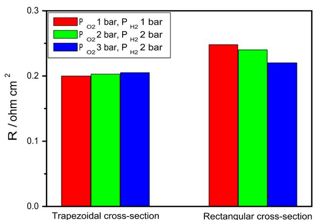
**Fig. 11 – Histogram of the ohmic resistance of PEMFCs with serpentine channels having rectangular and trapezoidal cross-section at various oxygen and hydrogen pressures.  $T_c/T_{hc}/T_{ha} = 80/85/95$  °C. PTFE content in the cathode MPL: 15 wt%.**
