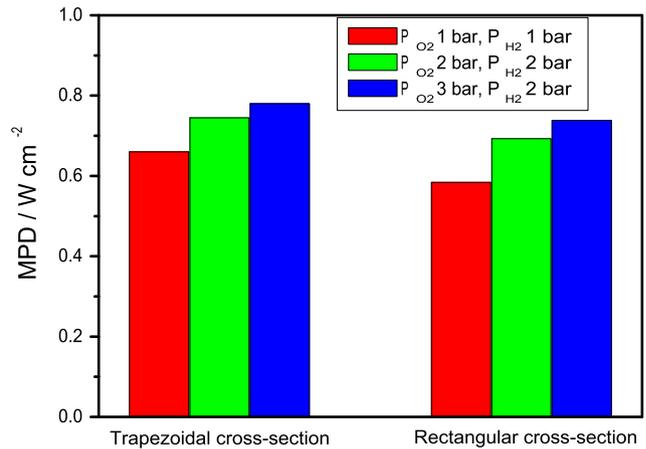
**Fig. 10** – Histogram of the maximum power density of PEMFCs with serpentine channels having rectangular and trapezoidal cross-section at various oxygen and hydrogen pressures.  $T_c/T_{hc}/T_{ha} = 80/85/95$  °C. PTFE content in the cathode MPL: 15 wt%.
