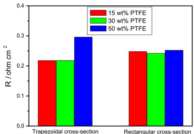
**Fig. 14** – Histogram of the ohmic resistance of PEMFCs with serpentine channels having rectangular and trapezoidal cross-section at various PTFE content in the cathode MPL.  $P_{O_2} = P_{H_2} = 1$  bar.  $T_c/T_{hc}/T_{ha} = 80/85/95$  °C.
