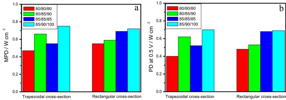
**Fig. 8** – Histogram of the maximum power density (a) and power density at 0.5 V (b) of PEMFCs with serpentine channels having rectangular and trapezoidal cross-section at various  $T_c/T_{hc}/T_{ha}$  conditions.  $P_{O_2} = P_{H_2} = 1$  bar. PTFE content in the cathode MPL: 15 wt%.
