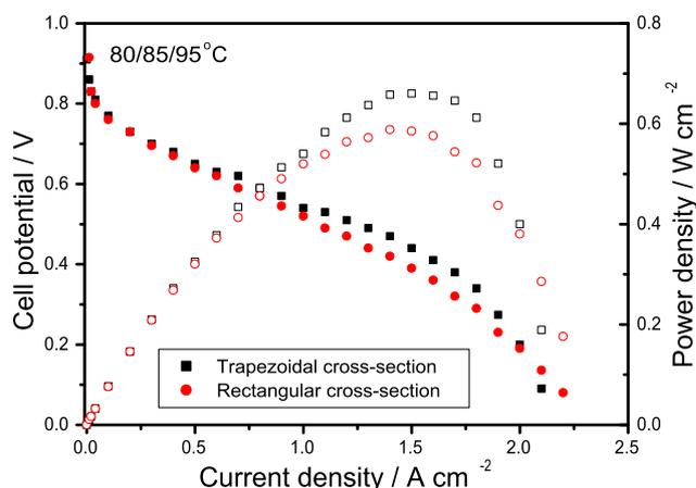
**Fig. 3 – Polarization and power density curves of single PEMFCs with serpentine channels having rectangular and trapezoidal cross-section.  $T_c$ : 80 °C;  $T_{hc}$ : 85 °C;  $T_{ha}$ : 95 °C; O<sub>2</sub> pressure: 1 bar; H<sub>2</sub> pressure: 1 bar; PTFE content in both anode and cathode MPL: 15 wt%. Anode and cathode catalyst: 20 wt% Pt/C, Pt loading 0.4 mg cm<sup>-2</sup>. Full symbols: polarization curves; open symbols: power density curves.**
