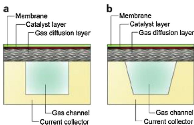
Fig. 2 – Cross-sectional views of flow channel geometries. (a): rectangular; (b): trapezoidal.
