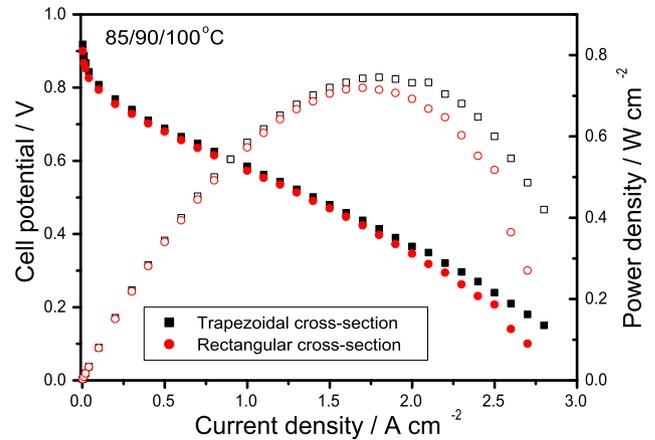
**Fig. 6** – Polarization and power density curves of single PEMFCs with serpentine channels having rectangular and trapezoidal cross-section.  $T_c$ : 85 °C;  $T_{hc}$ : 90 °C;  $T_{ha}$ : 100 °C;  $O_2$  pressure: 1 bar;  $H_2$  pressure: 1 bar; PTFE content in both anode and cathode MPL: 15 wt%. Anode and cathode catalyst: 20 wt% Pt/C, Pt loading 0.4 mg cm<sup>-2</sup>. Full symbols: polarization curves; open symbols: power density curves.
