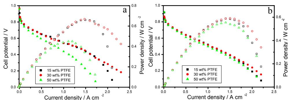
**Fig. 12 – Polarization and power density curves of single PEMFCs with serpentine channels having trapezoidal (a) and rectangular (b) cross-section with different PTFE content in the cathode MPL.  $T_c$ : 80 °C;  $T_{hc}$ : 85 °C;  $T_{ha}$ : 95 °C; PTFE content in both anode and cathode MPL: 15 wt%. Anode and cathode catalyst: 20 wt% Pt/C, Pt loading  $0.4 \text{ mg cm}^{-2}$ . Full symbols: polarization curves; open symbols: power density curves.**
