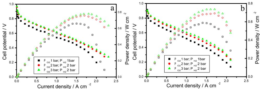
**Fig. 9** – Polarization and power density curves of single PEMFCs with serpentine channels having trapezoidal (a) and rectangular (b) cross-section at different oxygen and hydrogen pressures.  $T_c: 80$  °C;  $T_{hc}: 85$  °C;  $T_{ha}: 95$  °C; PTFE content in both anode and cathode MPL: 15 wt%. Anode and cathode catalyst: 20 wt% Pt/C, Pt loading 0.4 mg cm<sup>-2</sup>. Full symbols: polarization curves; open symbols: power density curves.
