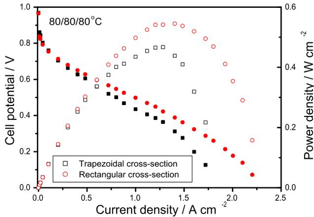
**Fig. 4** – Polarization and power density curves of single PEMFCs with serpentine channels having rectangular and trapezoidal cross-section.  $T_c$ : 80 °C;  $T_{hc}$ : 80 °C;  $T_{ha}$ : 80 °C;  $O_2$  pressure: 1 bar;  $H_2$  pressure: 1 bar; PTFE content in both anode and cathode MPL: 15 wt%. Anode and cathode catalyst: 20 wt% Pt/C, Pt loading 0.4 mg cm<sup>-2</sup>. Full symbols: polarization curves; open symbols: power density curves.
