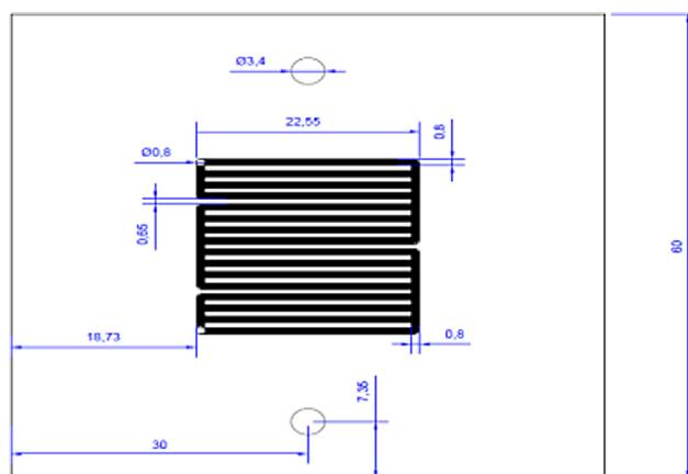
Fig. 1 – Serpentine flow field pattern.
