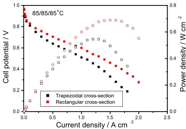
**Fig. 5** – Polarization and power density curves of single PEMFCs with serpentine channels having rectangular and trapezoidal cross-section.  $T_c$ : 85 °C;  $T_{hc}$ : 85 °C;  $T_{ha}$ : 85 °C;  $O_2$  pressure: 1 bar;  $H_2$  pressure: 1 bar; PTFE content in both anode and cathode MPL: 15 wt%. Anode and cathode catalyst: 20 wt% Pt/C, Pt loading 0.4 mg cm<sup>-2</sup>. Full symbols: polarization curves; open symbols: power density curves.
