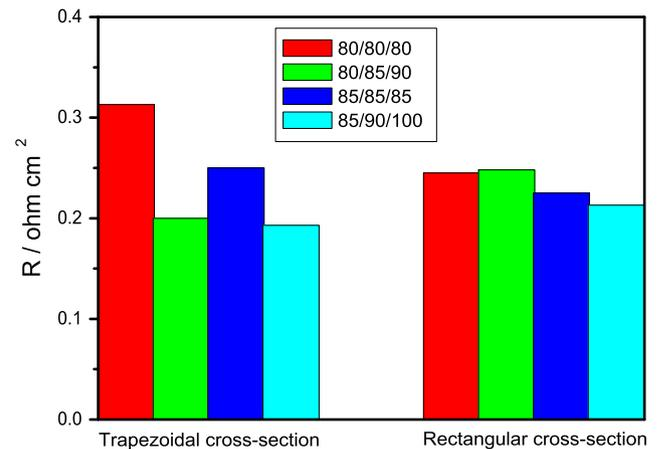
**Fig. 7** – Histogram of the ohmic resistance of PEMFCs with serpentine channels having rectangular and trapezoidal cross-section at various  $T_c/T_{hc}/T_{ha}$  conditions.  $P_{O_2} = P_{H_2} = 1$  bar. PTFE content in the cathode MPL: 15 wt%.
