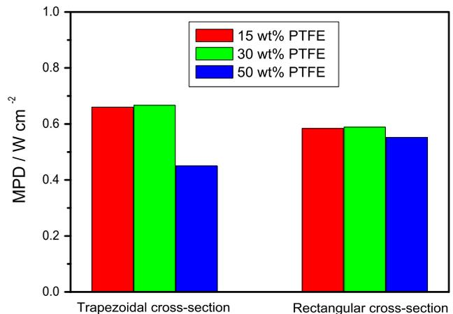
**Fig. 13** – Histogram of the maximum power density of PEMFCs with serpentine channels having rectangular and trapezoidal cross-section at various PTFE content in the cathode MPL.  $P_{O_2} = P_{H_2} = 1$  bar.  $T_c/T_{hc}/T_{ha} = 80/85/95$  °C.
