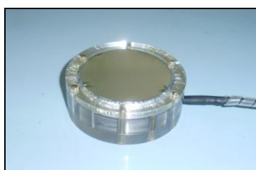
Fig. 1. Parallel plate ionization chamber studied in this work in beta radiation standard fields.
