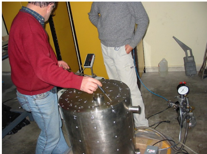
Fig. 11. Helium leakage test.
