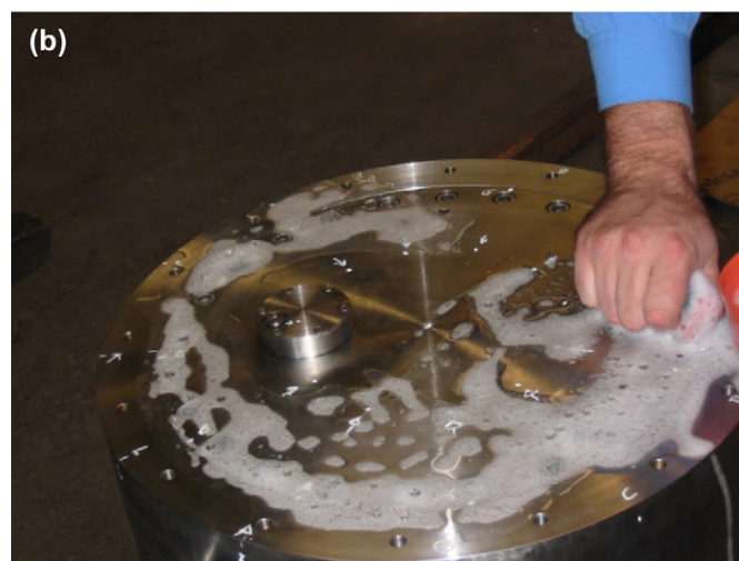
Fig. 12. Pneumatic pressure test.
