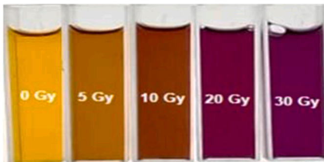
Fig. 3. Photograph of disposable acrylic cuvettes with non-irradiated (0 Gy) and irradiated FXG solutions with 5, 10, 20 and 30 Gy (from left to right).
