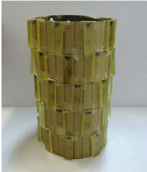
Fig. 1. Arrangement of the PC dosimeters for field mapping in the cylindrical container in Gammacell 220.
