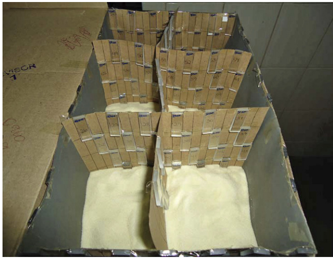
Fig. 2. Arrangement of the PC dosimeters for field mapping in the parallelepiped container irradiated with the panoramic Co-60 source.
