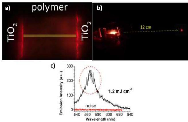
Figure 1: a) Image of the polymer strip with TiO<sub>2</sub> particles. b) Low divergence red laser emission of microfluidic RL. c) Persistent, localized modes on top of the ASE band of the extended modes, indicating suppression of the interaction between the localized modes.
