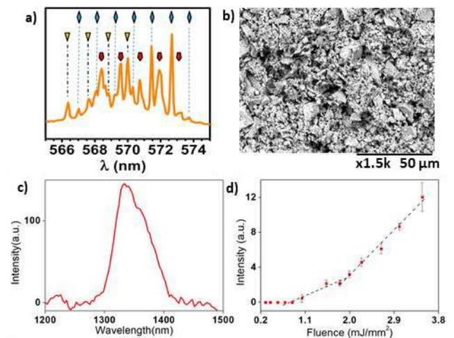
Figure 3: a) three sets of equidistant peaks with the same FSR corresponding to three resonators of the same length within the pump spot size. b) image of the random laser surface. c) emission at 1337 nm. d) output power versus input power clearly showing two different slopes, the first attributed to cavity-enhanced coherent emission and the second to additional incoherent emission due to ASE or extended modes.
