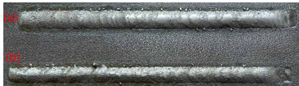
Figure 3. Images of iron aluminide tracks deposited via laser cladding: (a) \text{Fe}_3\text{Al} track 4 and (b) FeAl track 6.
