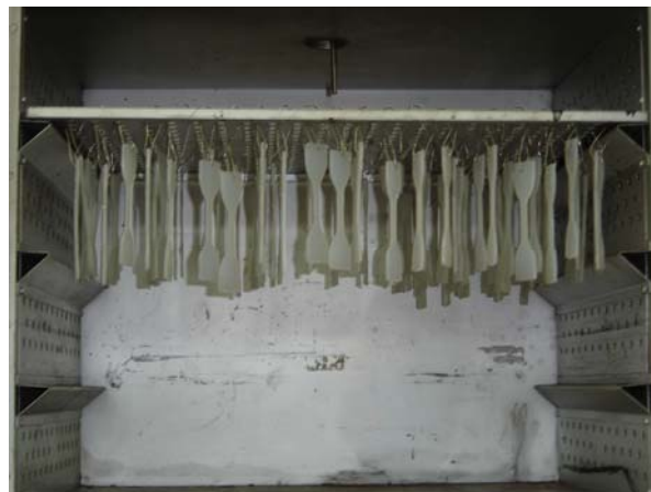
Figure 1 - The disposal to the samples of the PP and HMS-PP inside of stove with air circulation, at the temperature of 90^\circ\text{C} .
