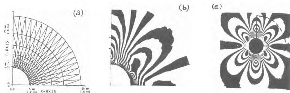
Figure 4 - Stress distribution around a hole (Weathers et al. 1985).
