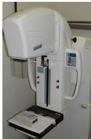
Figure 5. Diavolt placed 60 cm away from the focal spot (mammograph)
