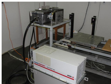
Figure 1. Industrial System Pantak/Seifert (constant potential)
