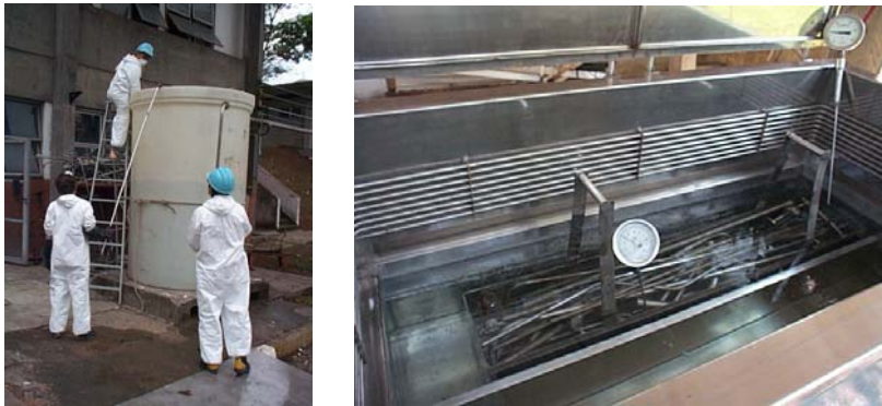
Figure 3: Immersion tank and ultrasonic equipment used for decontamination.
