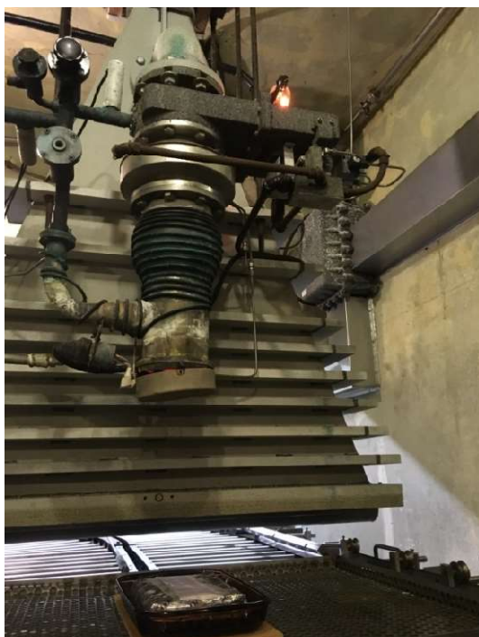
Figure 1: EB arrangement for paper samples irradiation, radiation absorbed dose of 25 kGy at low temperature (frozen foam ice).
