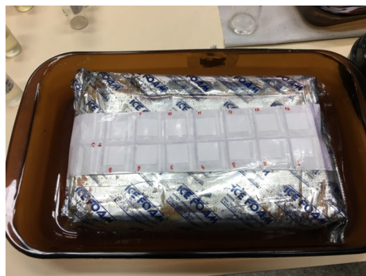
Figure 1: EB arrangement for paper samples irradiation, radiation absorbed dose of 25 kGy at low temperature (frozen foam ice).
