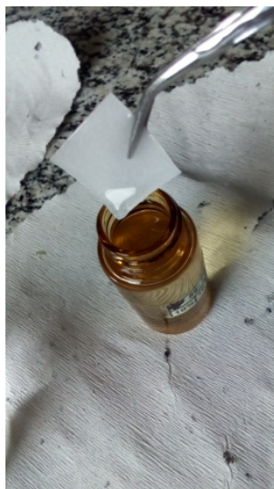
Figure 5: Simultaneous method of grafting of NVP onto cellulose in ethanol:water 25:75 v:v solution, using gamma radiation: (A) 0 %, 5 %, 10 % and 20 % NVP, left to right; (B) 10 % NVP and (C) 20 % NVP.
