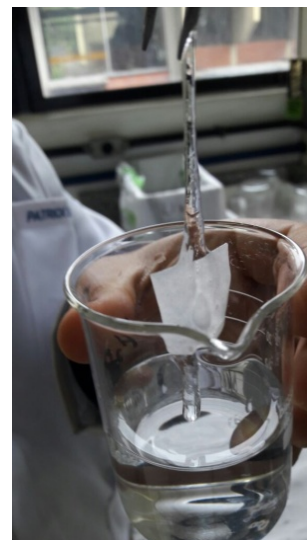
Figure 5: Simultaneous method of grafting of NVP onto cellulose in ethanol:water 25:75 v:v solution, using gamma radiation: (A) 0 %, 5 %, 10 % and 20 % NVP, left to right; (B) 10 % NVP and (C) 20 % NVP.
