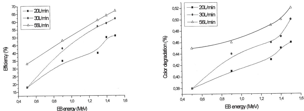
Fig. 4. Efficiency of the irradiation device and the colour dye degradation as a function of electron beam energy.
