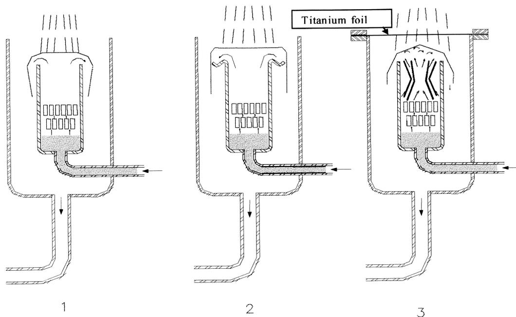
Fig. 1. Models of up-flow stream irradiation devices.
