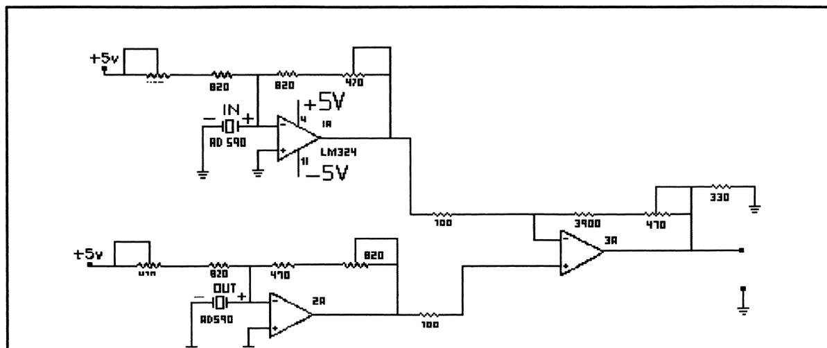
Fig. 3. Dosimetric system electric circuit diagram.
