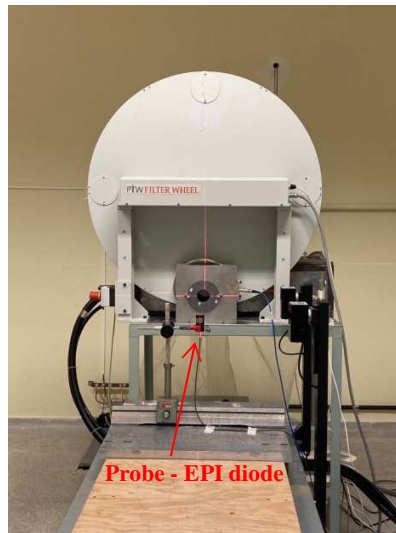
Figure 1: Probe of the EPI diode set at Pantak-Seifert 160HS Isovolt X-ray generator.
