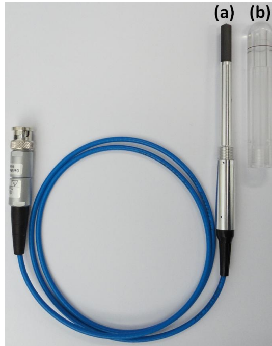
Figure 2. Commercial ionization chamber (a) PTW Farmer, model TN30011-1, and (b) its build-up cap.
