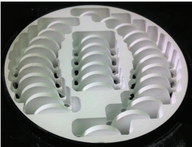
Figure 1 - Illustrative image of the pre-sintered Y-TZP discs milled with CAD-CAM technology
