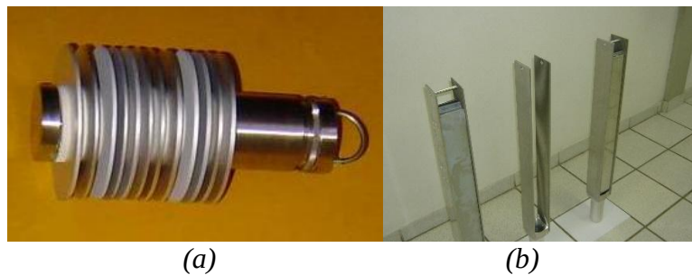
FIG. 1. Photographs of: (a) coupons stacked in a rack; (b) plates assembled to form dummy fuel elements.
