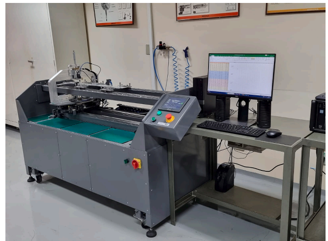
Fig. 5. General view of the equipment for automated measurement of nuclear fuel plates.
