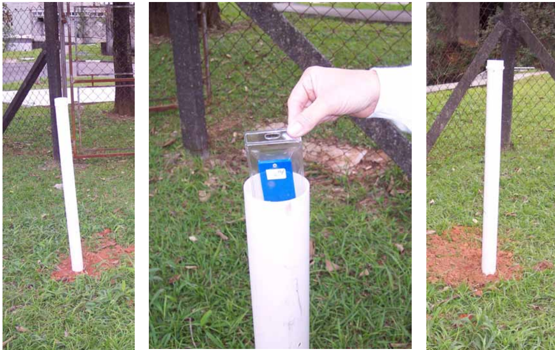
Figure 1: Illustration of the stack pole arrangement used as holder for single dosimeter 1m above ground.
