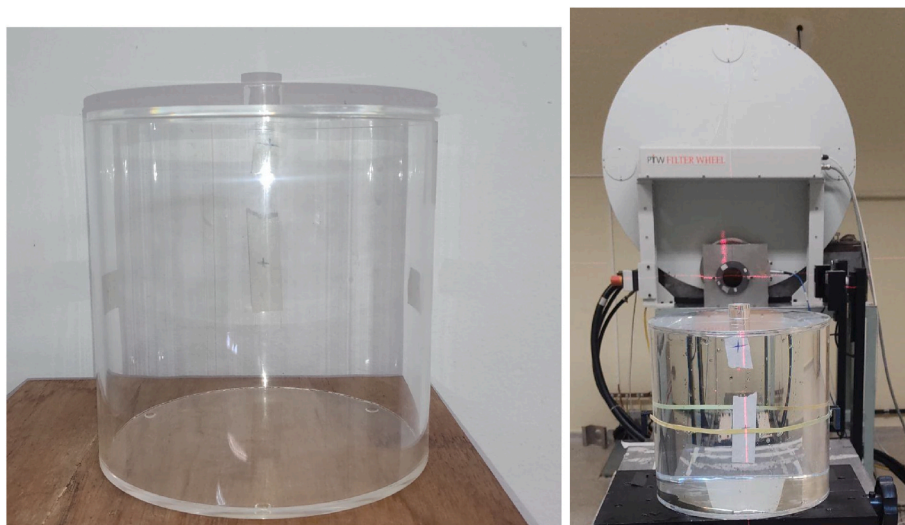
Fig. 6. (a) Phantom recommended by ICRU, (b) Arrangement for irradiation in the standard ICRU phantom.
