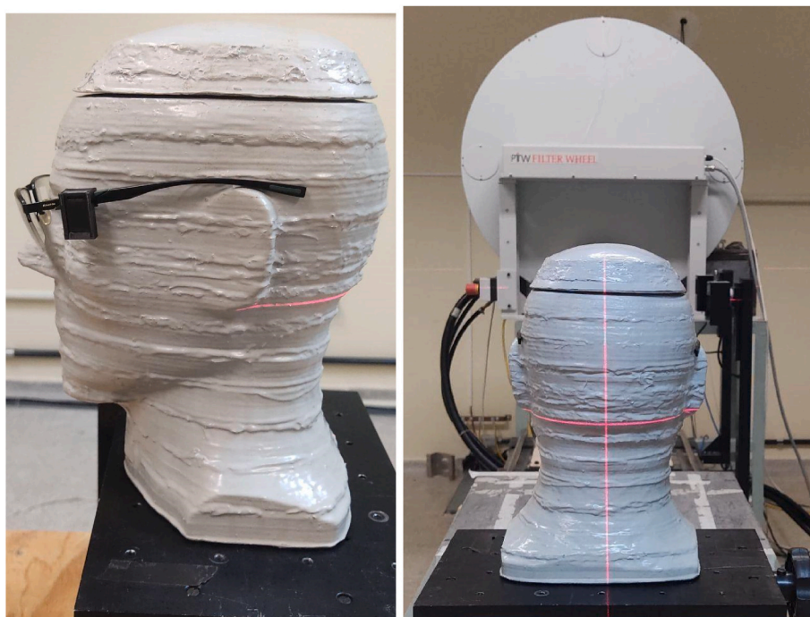
Fig. 7. (a) Phantom anthropomorphic, (b) Arrangement for irradiation in the anthropomorphic phantom.
