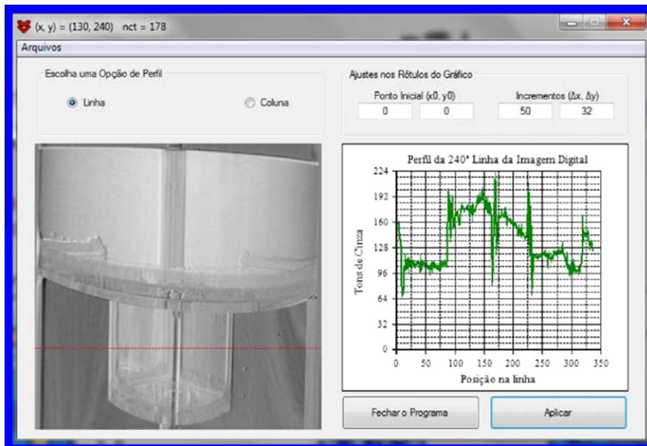
Fig. 5. Processed image of the lower region of the ST – ( $t = 2$  h).
