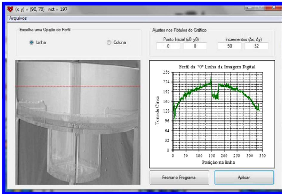
Fig. 4. Processed image of the upper region of the ST – ( $t = 2$  h).
