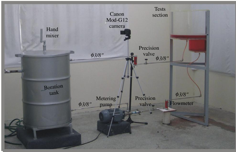
Fig. 3. Device used for acquiring the pictures and videos during the experiments.
