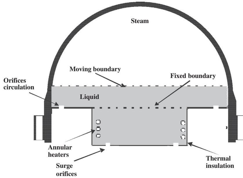
Fig. 1. Transversal cut of the IRIS pressurizer.
