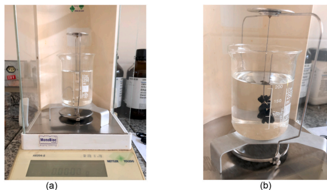
Fig. 2. Kit 33360 Mettler Toledo (Archimedes principle)- ASTM D3800.
