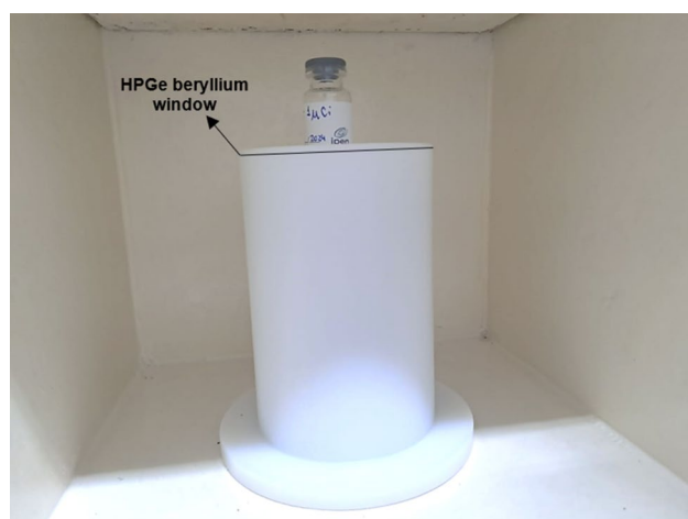
Fig. 4 - Geometry used for analysis in the detector HPGe
