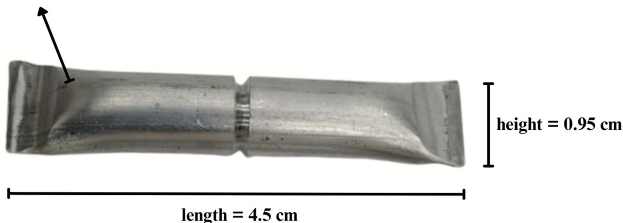
Fig. 2 Aluminum capsule for containing Xe gas
