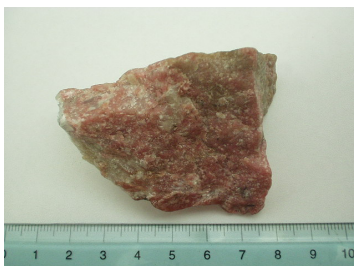
Figure 1. Natural rhodonite used for the production of rhodonite-Teflon pellets.
