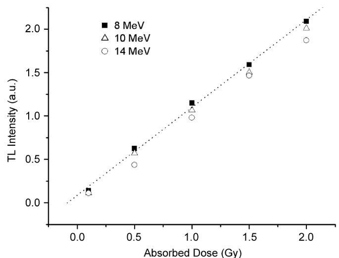
Fig. 3. Pure LiF dose response to electrons beams.
