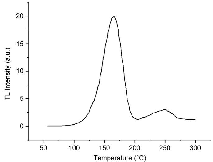
Fig. 1. Typical TL glow curve of a pure LiF detector exposed to electron beams (5 Gy, 10 MeV).
