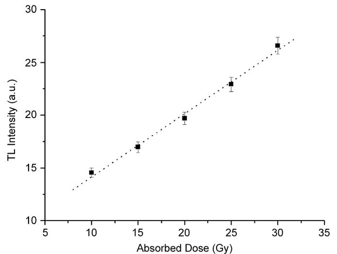
Fig. 2. Pure LiF dose response to gamma radiation.
