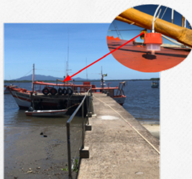
Figure 3: Vessel IOUSP, in highlight the position inlet of portable gas analyzer
