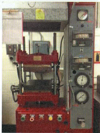
FIG. 2.4. Hot press used to manufacture nanocomposites at University of Dayton.
