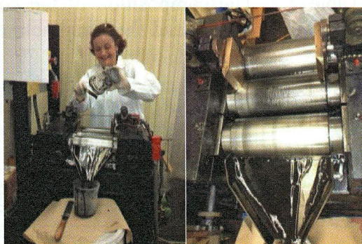
FIG. 2.2. Three roll mill dispersion at composites carried out at University of Dayton Lab.
